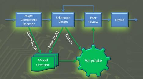
Valydate's Schematic Integrity Analysis is performed in parallel with your design and does not affect the schedule of your hardware development (Except for saving you time during lab testing and debugging!).
